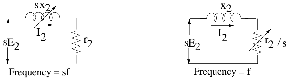
(a) Rotor circuit of the actual motor (b) Rotor circuit of the fictitious motor
