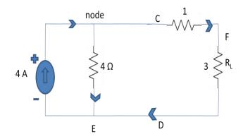
So, 4A current is divided into two equal parts at node because each of the two parallel paths has a resistance of 4  $\Omega$ . I<sub>RL</sub>= 2 A.
