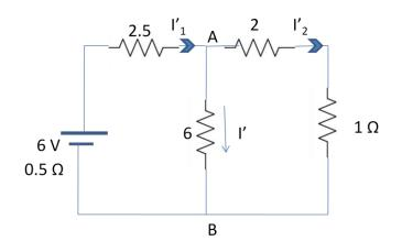
Here only 6 V is considering by removing 12 V with its internal resistance of 1  $\Omega$ .
