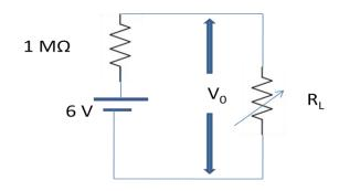
6 V battery has an internal resistance of 1 M $\Omega$  and load resistance varies between 20 K $\Omega$  to 200 K $\Omega$ . So, current supplied by the source varies from 6/1.02 = 5.9  $\mu$ A to 6/1.2 = 5  $\mu$ A. So, it is seen that even when load resistance increases 10 times, current decreases by 0.9  $\mu$ A. Hence source can be considered constant current source.
