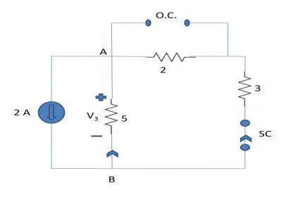
Current 2 A divides equally at point B, because the two parallel paths have equal resistance of 5  $\Omega$  each.
