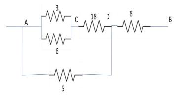
**Solution**: Resistance between A and C= 6 ||  $3 = \frac{6X3}{6+3} = 2\Omega$
