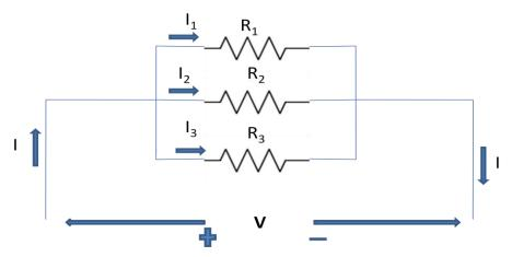
Fig 7 parallel connection of resistances
