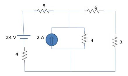
**Solution**: First of all we have to convert 2 A current source and parallel resistance to a voltage source with series resistance by source conversion technique and redraw the circuit.
