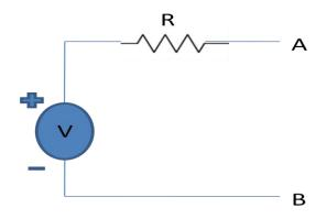
Fig.16(a) Voltage source with series resistance
