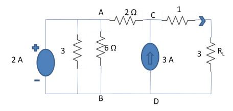
The two parallel resistances of  $3\Omega$  and  $6\Omega$  can be converted into equivalent resistance of  $2\Omega$ .
