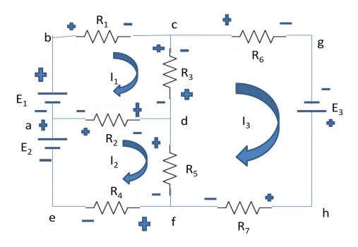
Fig.20 Mesh analysis of a circuit
