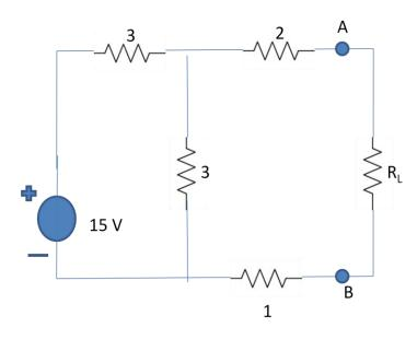
**Solution:** First remove  $R_L$  to find the equivalent Thevenin's source of the circuit to the left of terminals A and B.
