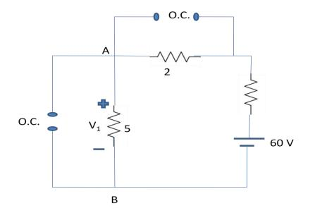
$V_1 = 60 \times \frac{5}{5+2+3} = 30 V$ ; its value is taken positive, because current through the 5  $\Omega$  resistor from A to B, so making the upper end of resistor positive and the lower end negative.
