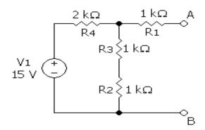
Solution:  $V_{\text{Th}} = \frac{R_2 + R_3}{(R_2 + R_3) + R_4} \cdot V_1 = \frac{1+1}{1+1+2}$  .15 = 7.5 V
