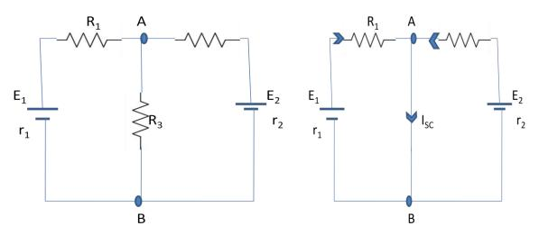
$I_{SC} = \frac{E_1}{R_1} + \frac{E_2}{R_2} = E_1 G_1 + E_2 G_2$
