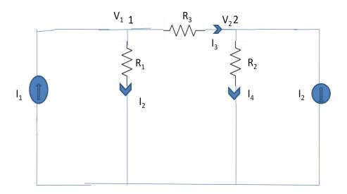
Fig.23 Node Voltage Analysis with Current Sources
