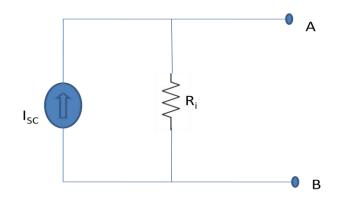
Fig.25 Norton equivalent circuit
