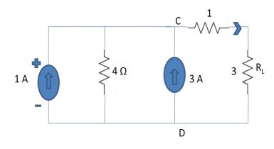
Here, there are two current sources 1A and 3A entering into a node and leaving through CE and CFD path like below, then we can apply KCL here to find out current through  $R_L$ . So,
