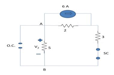
In the above figure, the 6 A current source has two parallel circuit across it; one having the resistor of 2 $\Omega$  and other path having the series connection of resistances  $(3+5) = 8 \Omega$ . Using the current divider rule, the current through 5  $\Omega$  resistor=  $6 \times \frac{2}{(2+3+5)} = 1.2 \text{ A}$
