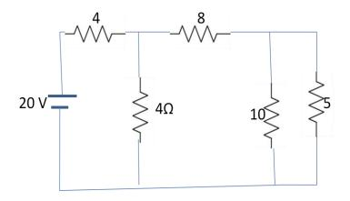
**Solution:** Remove 5  $\Omega$  resistor and put short circuit across it.
