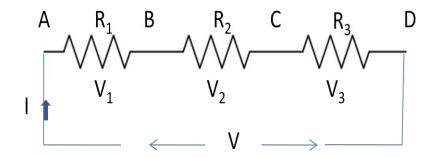
Fig 6 Series connection of resistances
