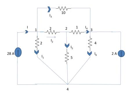
**Solution**: Node 1: V<sub>1</sub>  $(\frac{1}{2} + \frac{1}{2} + \frac{1}{10}) - \frac{V_2}{2} - \frac{V_3}{10} = 8$
