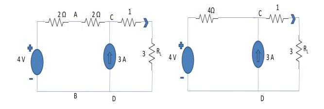
In the above figure, you can see that there is a series connection of 4V voltage source and  $4\Omega$  resistance. So, it can be converted into equivalent current source of 1A with parallel resistance of  $1\Omega$ .
