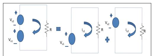
According to superposition theorem, one source should be present at a time, deactivating remaining sources. Contributions due to individual sources are finally algebraically added to get the final answer.
