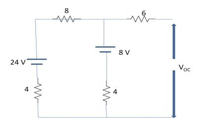
For finding  $V_{OC}$ , net voltage= 24- 8= 16 V
