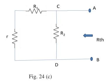
$$R_{th} = R_2 \parallel (R_1 + r) = \frac{R_2 (R_1 + r)}{R_1 + R_2 + r}$$
