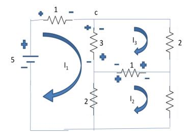
**Solution**: In mesh-1, mesh equation is  $6I_1 - 2I_2 - 3I_3 = 5$
