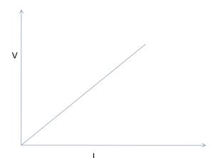
Fig.5 The V-I characteristic of resistance
