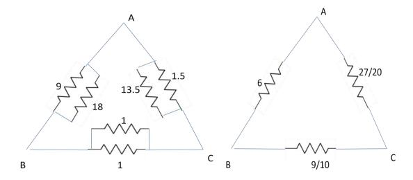
$R_{AB}$  is the resistance between terminals A and B means 6 || (27/20+ 9/10),  $R_{BC}$  is the resistance between terminals B and C i.e. 9/10 || (6+ 27/20) and  $R_{CA}$  is the resistance between terminals C and A i.e., 27/20 || (6+ 9/10).
