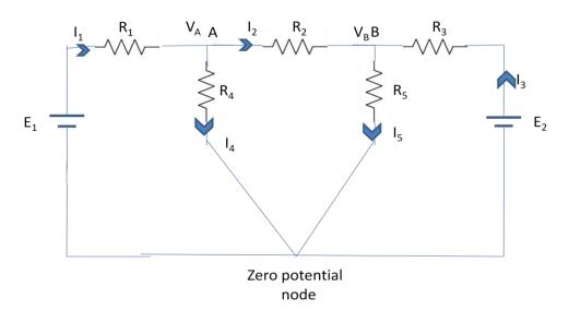
Fig.21 Node voltage Analysis
