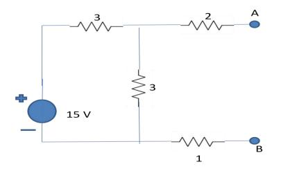
$V_{th}$  is equal to the drop across 3  $\Omega$  resistor because no current will flow through 2  $\Omega$  and 1  $\Omega$ .
