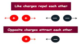
Fig. 1: The behavior of likely charged and unlikely charged atoms.
