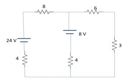
We have to find out current flowing through 3  $\Omega$  resistor. According to Thevenin's theorem, we have to remove that resistor whose current is required. So, 3  $\Omega$  resistor has to be removed from the circuit. After removing, the new circuit is as follows.
