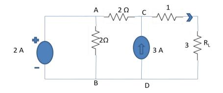
Now, the 2A current source with parallel resistance 2  $\Omega$  can be converted into equivalent 4V voltage source with 2 $\Omega$  series resistance. Again, the series connection of two 2 $\Omega$  resistance can be converted into one 4 $\Omega$  resistance.
