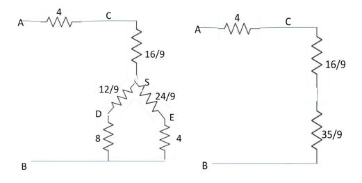
The two parallel path between S and B can be reduced to a single resistance of 35/9 i.e.,  $(12/9 + 8) \parallel (24/9 + 4)$ .
