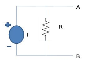
Fig.16(c) Current source with parallel resistance
